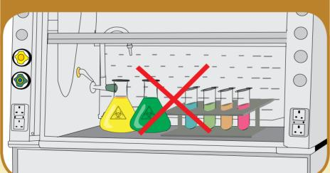
If performance is suspect or an airflow alarm is triggered (if installed), terminate usage, close the sash completely and cease work
