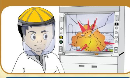
If a combination sash is installed, do not open the vertical and horizontal sashes simultaneously
