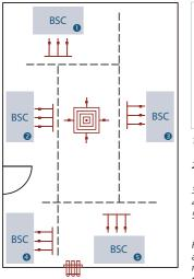
Fig 7. A Typical Class II Cabinet Installation
