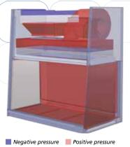
The Esco double-wall design creates a Dynamic Chamber plenum which surrounds contaminated areas with negative pressure, preventing the possibility of contamination from leaks in filter seal, gasket or cabinet structure.
