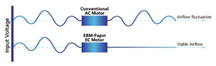
The Esco NordicSafe uses latest generation EBM-Papst EC Motor (ECM) to maintain stable airflow despite building voltage fluctuations, thereby assuring constant face velocity and downflow for optimum safety, containment and protection.
